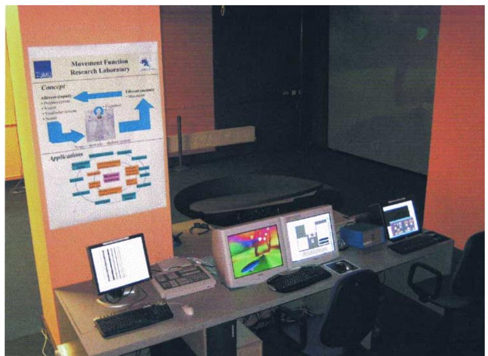
**Figure 2: The layout of the laboratory. A local network of computers controls the Vicon 612 and the virtual reality components including the movable platform and 3D video.**
