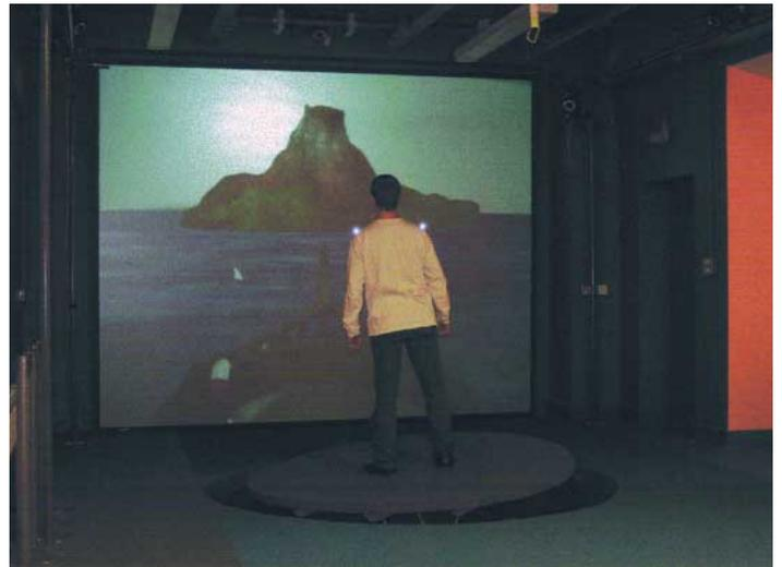
*Figure 4: In the "Boat" environment the underlying logic can be described by real time feedback loops. The subject's movement drives the boat on the 3D video screen and the platform responds at the same time. The feedback is that the movement of the platform has an effect on the subject's balance.*
