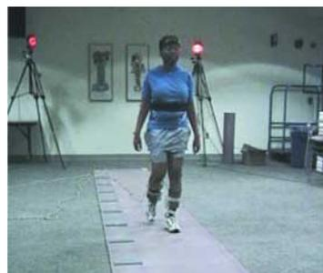
Figure 2b. The experiment subject wearing a dual-axis AFO which allows relatively "normal" kinematic function compared to plastic posterior leaf spring design AFOs.
