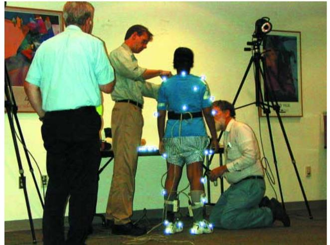
Figure 2a. Placement of photoreflective markers on an experimental subject in a comparative gait trial evaluating the kinematics of ankle foot orthoses.
