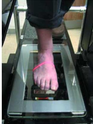
**Figure 3b. 3-D digitization of an experiment subject's foot and ankle with the VA Pedorthics Optical Digitizer.**
