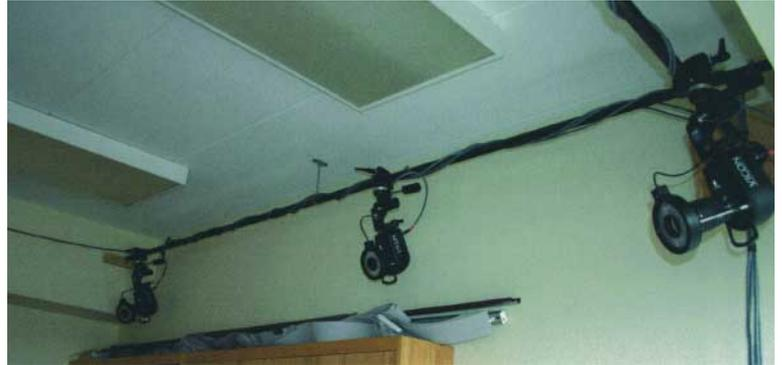
Figure 1 Adjustable Vicon permanent camera mounts in small volume capture laboratory.
